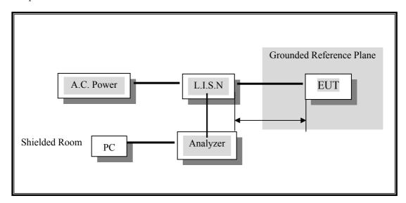
The EUT is on an insulating plane (height=80cm)
